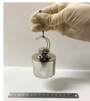
Photo 3. CNT yarn of φ0.4 mm capable of lifting a load of 1 kg
